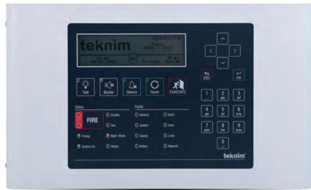
Teknim TFP-1240 repeater panel is developed to monitor and intervene fire detection systems from different points at large and medium scale enterprises. It can be connected approximately up to 1.000 meters distance from main panel over RS-485 communication layer. Slim and aesthetic design fits into any office environment, guard kiosk, recep-
